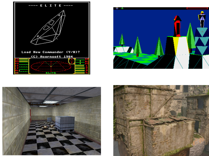
Figure 3: Top Left: Wireframe Graphics, Elite 1984 ; Top Right: Coloured Polygons, Sentinel 1986 ; Bottom Left, Textured Polygons: Half-Life 1998 ; Bump Mapping, Shaders, Uncharted 4, 2016
